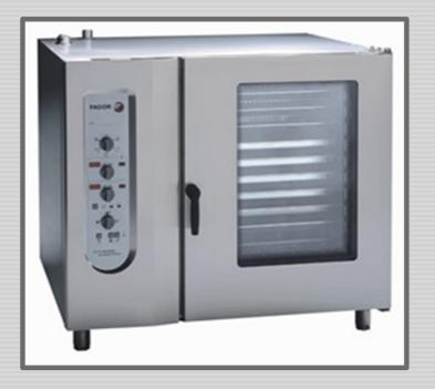
Built-in high-yield steam generator with system to detect calcareous depositions. Safety thermostat. Time selector. Digital control panel. Core probe. Door safety switch for the opening. Flue equipped with opening & closing device. Stainless steel burner with electronic control system. Door with double folding glass toward the interior & hermetic locking. Shower tap for the cleaning. Available in propane gas, natural gas and electric 5 cooking modes:
