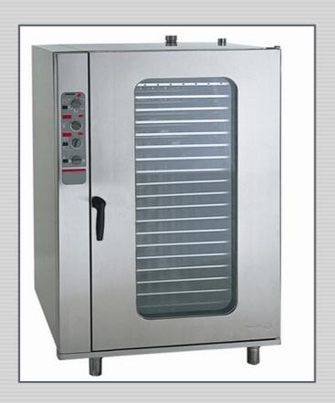
Built-in high-yield steam generator with system to detect calcareous depositions. Safety thermostat. Time selector. Digital control panel. Core probe. Door safety switch for the opening. Flue equipped with opening & closing device. Stainless steel burner with electronic control system. Door with double folding glass toward the interior & hermetic locking. Shower tap for the cleaning. Available in propane gas, natural gas and electric 5 cooking modes:
