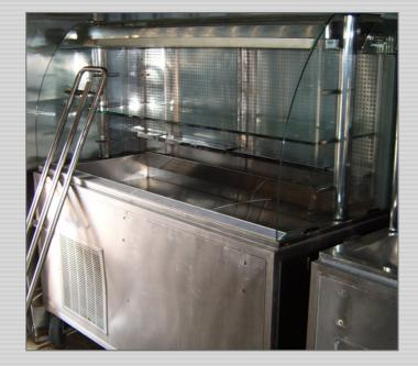
High quality stainless steel2 x glass display shelves4 x heavy duty casters 2 with brakesTray slide availableLoading doors from the rear
