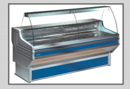
Refrigerated under storage Intermediate glass shelf Marble rear shelf Stainless steel deck Digital controller Digital temperature readout Temperature range +0 C to +5 C Suitable for 25 C ambient temperature Fan assisted
