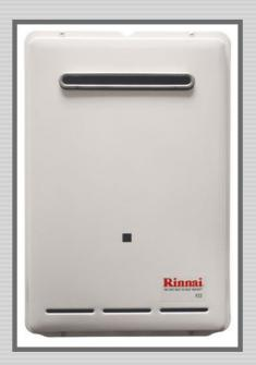
The Rinnai Twin Flow features a unique flow switch which regulates the maximum gas loading for the system. At 6 litres/min (domestic hot water flow rate) and above the boiler automatically switches to standby, allowing the water heater to operate at maximum capacity. This eliminates the need for a larger gas supply or metering.
