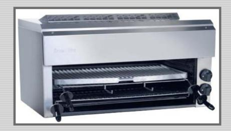
Stainless steel sides and top, Stainless steel control panel, Vitreous enamelled interior for easy cleaning Surface combustion plaque burner with low turn down facility, Flame failure device on burner, removable grease trough, reversible ribbed brander plate (also reversible), adjustable height toast rack and crumb tray
